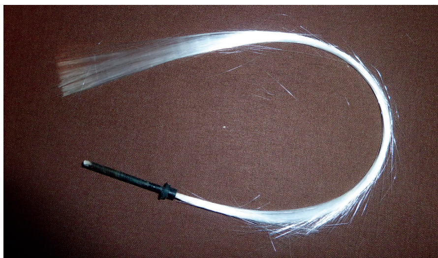
Figure 2: A bundle of early optical fibres each narrower than a human hair.
