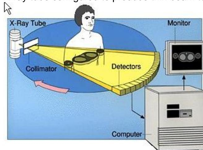
X-ray tube and detector array housed within gantry which can rotate 360 degrees around patient.
